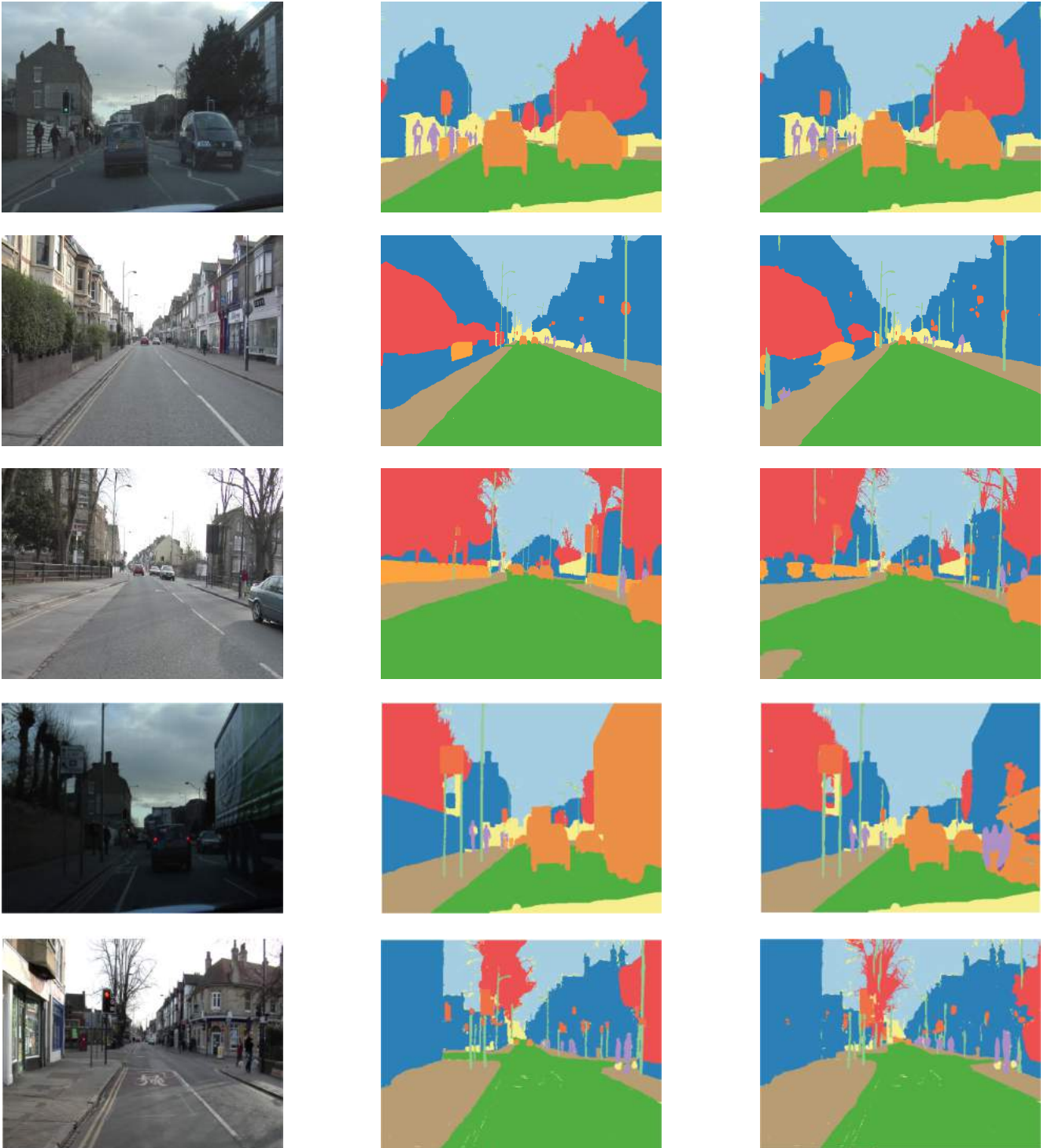
Figure 3. Qualitative results on the CamVid test set. Pixels labeled in yellow are void class. Each row represents (from left to right): original image, original annotation (ground truth) and prediction of our model.
