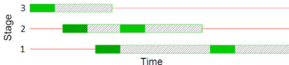
Figure 2-1: Actuated control dynamics
