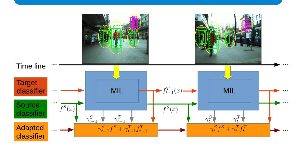
Incremental domain adaptation framework.  $f_t^T(x)$  is the classifier trained in a multiple instance learning (MIL) manual with current target image, while the final target-domain adapted classifier is:  $\gamma_t^S f^S(x) + \gamma_t^T f_t^T(x)$
