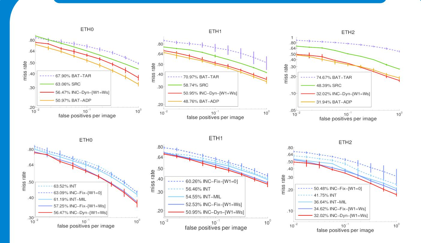
Results of adapting a DPM pedestrian detector trained with synthetic images to operate in ETH pedestrian dataset.
